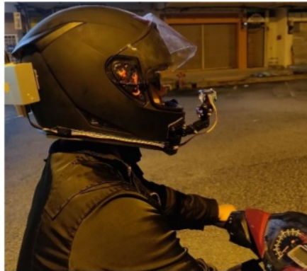
Figure 8. The rider with NAVHELM is able to get navigation information without looking down
