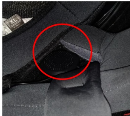
Figure 9. NAVHELM implement speaker inside the helmet to provide audio navigation
